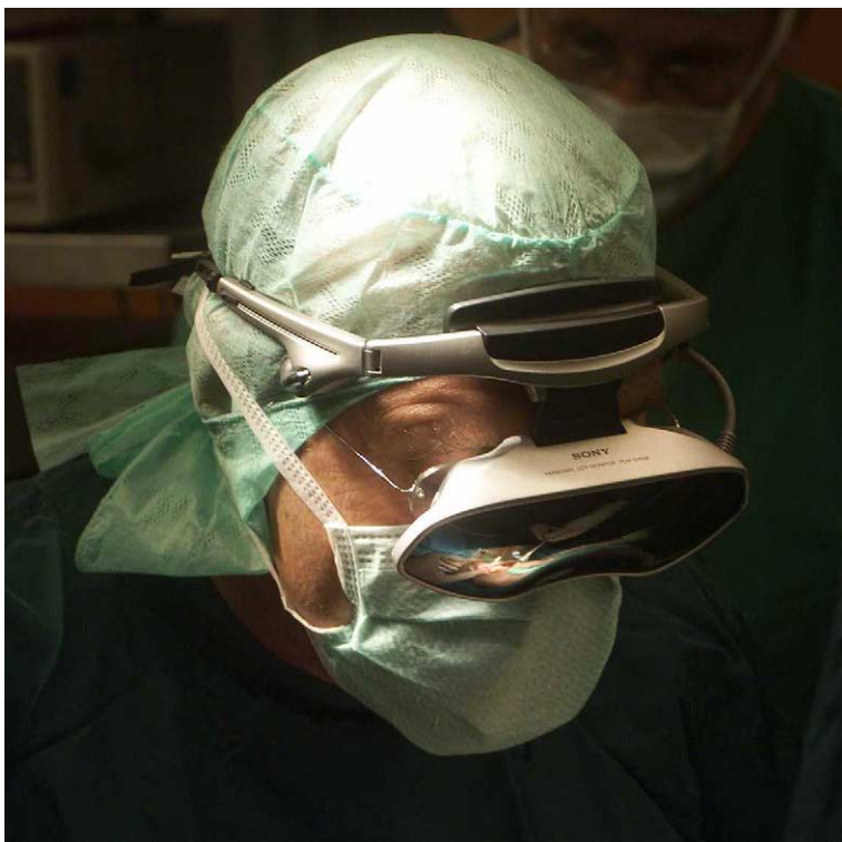
Fig. 5. Glasses with LCD-displays enable the surgeon to “receive” the information from the preoperative planning in the surgical field intraoperatively.
