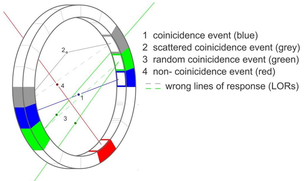
Figure 11. **Types of coincidence detections**
