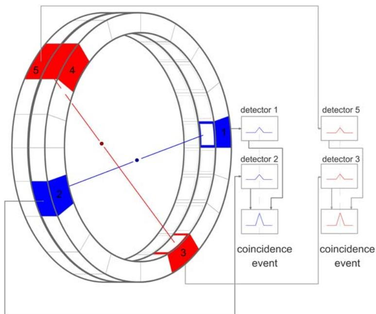
Figure 12. **Principle of a 3D PET camera**
