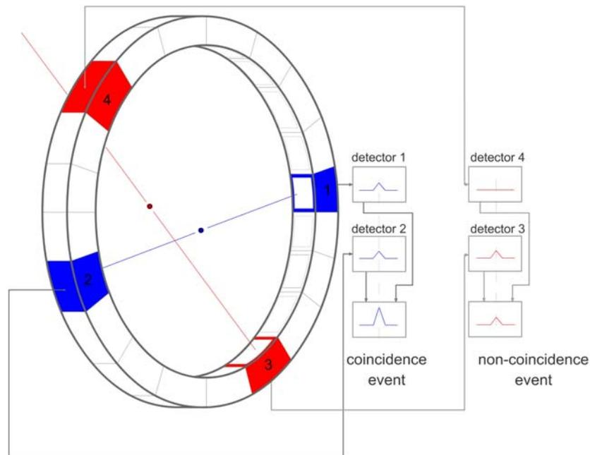
Figure 10. **Coincidence detection of gamma rays in PET (2D mode)**
