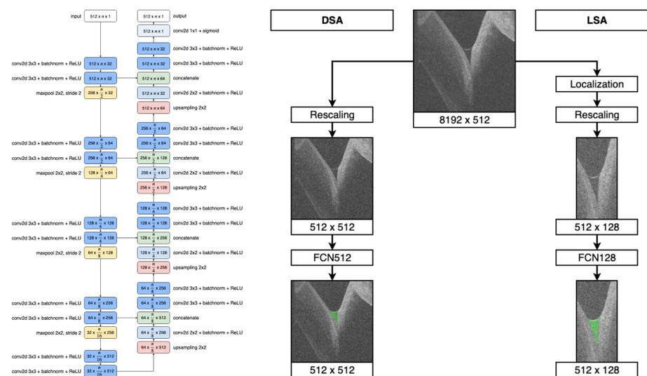
Fig. 3 - Left: U-Net-like architectures of the segmentation networks, which only differ in their input dimension  $n$ . Right: Segmentation workflow of the two compared approaches. For FCN512,  $n=512$  and for FCN 128,  $n=128$ . [2]
