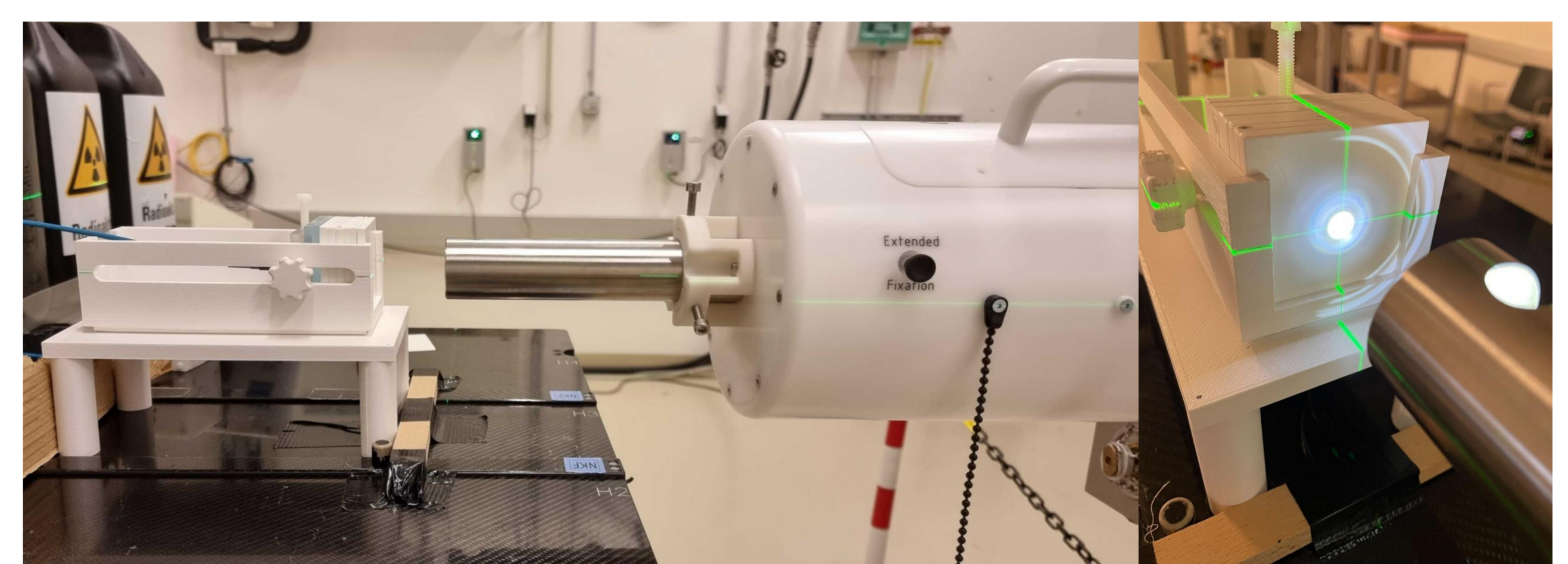
Figure 4: Proton beam dosimetry setup in two different views
